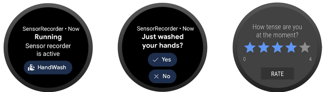
Fig. 2 Interface displayed on the smartwatch. The leftmost screenshot shows the default state. The application shows the user that a recording is running, and the button to annotate a hand wash event is displayed. The center screenshot shows the question displayed to the user after an automatic detection of a hand wash. The user can either confirm the hand wash by pressing “Yes”, or correct the detection by pressing “No”. The screenshot on the right shows the rating scale used to measure the urge to wash hands and the current distress of the user. The user could select values from 1 to 5 on the scale by tapping or sliding on the stars and confirming by pressing the “Rate” button.
