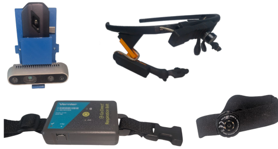
Figure 5: An overview of the hardware suite used for multi-modal data collection. The components are (clockwise from top left): the thermal (Topdon TC001) and depth (Intel RealSense) camera assembly; the Pupil Labs head-mounted eye-tracker; the Polar OH1 photoplethysmography (PPG) arm-band sensor; and the Vernier Go Direct Respiration Belt.
