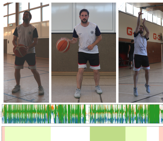
Figure 1: A basketball player while dribbling and shooting (top), the raw inertial sensor data (middle plot) with classified sequences (bottom plot).
