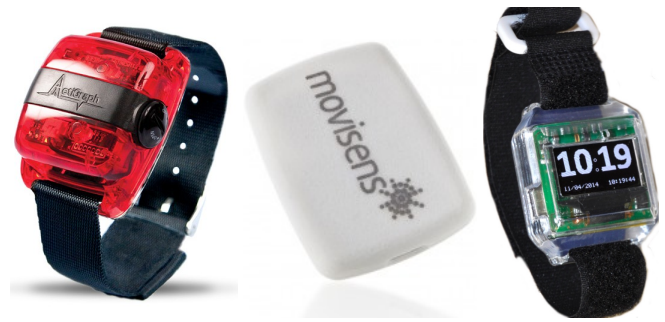
Figure 2. The participants' activities were monitored with a variety of accelerometer-based activity loggers (from left to right): the Actigraph GT3X, the Movisens move II, and the Hedgehog. All capture 3D acceleration at a frequency of 30 to 100 Hz for at least a week, continuously.
