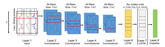
Figure 1: Illustration of the suggested change to the DeepConvLSTM [26] architecture. The change involves removing the second LSTM layer (Layer 7). During experiments we either include (original architecture) or exclude Layer 7 (our suggestion) and vary the amount of hidden units within the LSTM layer(s) (i.e. Layers 6 and 7) to be either 128, 256, 512 or 1024.
