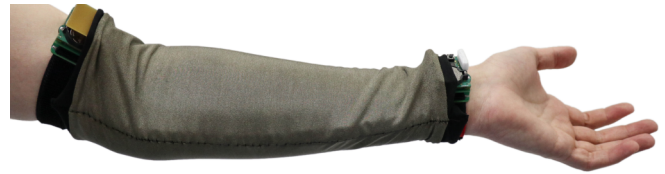
Figure 1. Our body-coupled communication approach uses the human body as a transmission medium for the signal path, with a nearby conductive fabric for a robust feedback path, between wearable units.
