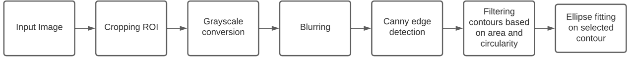
Figure 2: Our pupil detection pipeline, which is implemented in Python3 and makes extensive use of the OpenCV library [29], is made available open-source. It uses ellipse fitting, where the input image is capture in infrared lighting, and confidence on the parameter selection for canny ( T_{canny} ) and blurring ( K_{blur} ) is performed using the parameter estimation routine (sec 4.2).
