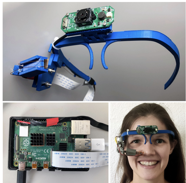
Figure 1: The 3D-printed hardware setup connects two cameras through USB and CSI, along a LED power delivery using GPIO to the Raspberry Pi Model 4 B. The bottom-right image shows the front view of the hardware while worn.
