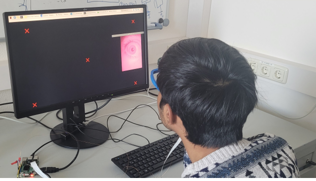
Figure 3: Study participants perform the experiments, while these run completely on the embedded system itself. The Raspberry Pi (left) acquires the images, while in the fixed marker location experiment each participant would start from the top left marker location, and would go to top right marker, followed by central marker, then bottom left marker, and finally bottom right marker. Displayed here are all markers and the real-time eye camera feed, which is not displayed to the participant while performing the experiment.
