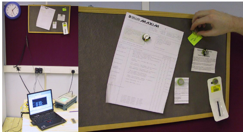
Fig. 5. The two layers of the board are connected to a computer (left), on which the software runs that acts as a master for the network. New documents can be added by pinning them in (right). A pin will start flashing its LED (see upper-left pushpin) when a document expires (i.e. when the pin's alarm flag is set) and no other expired documents have a higher priority.
