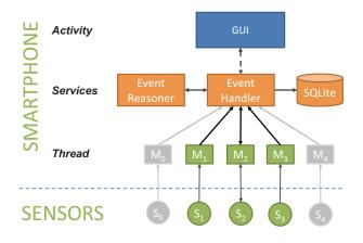
Figure 1: Layered, event-driven middleware architecture for body sensor networks providing high extendibility and adaptability as well as a seamless handling of sensor configuration changes.
