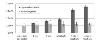
Figure 5: Energy consumption of myHealthAssistant and the Android system with different sensor configurations.
