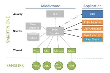
Figure 3: Implementation of *myHealthAssistant*: Application-specific modules send and receive events via the *EventHandler*. Sensor modules translate raw sensor data to events.
