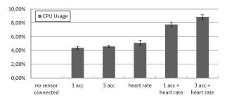
Figure 6: myHealthAssistant CPU utilization of different sensor configurations.
